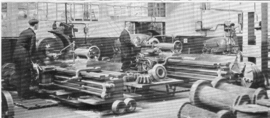
Fig. 25 (top)—Threading mixer discharge door screws on a 24 in. swing Lang centre lathe. The screws have a double start, \frac{1}{8} in. pitch \times 16 in. long.
