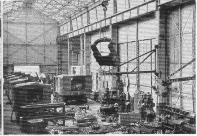
Figs. 87 & 88—Assembling a batch of Rapier 423 excavators. This bay is 42 ft. high to the eaves and is serviced by 25-ton and 15-ton overhead travelling cranes.
