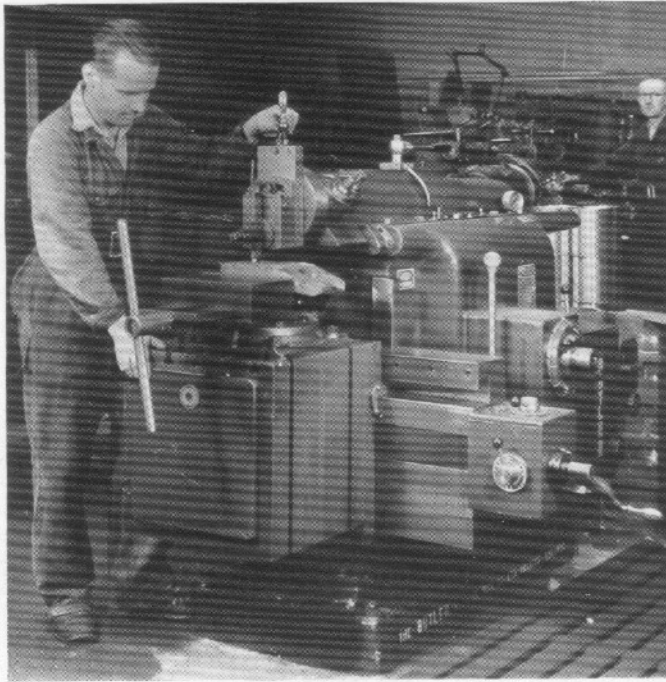
Fig. 51 (above)—Butler 18 in. stroke Super Shaper engaged on machining m.s. latch plates.
